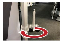
**Step 3.** Unscrew the pole pin wing nut, slide the pin through the accessory piece hole, and lock in place with the wing nut.
