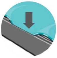
Fit graphic into corners, then "tap" into rest of frame channel.
