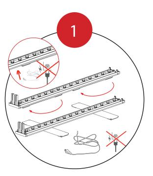
Fit the Bottom Extrusions together.
