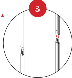
Fit the Top Extrusions together.
