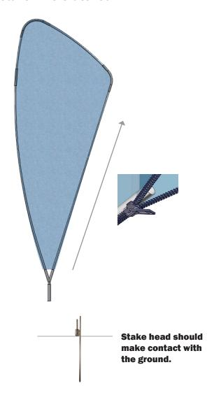
Fit unit onto inserted ground stake (mount on shorter pin).
