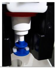
Never disassemble the nozzle portion of the pump mechanism, as taking this apart may cause irrepairable damage to your unit and cause it to leak.
