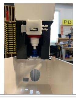
If your dispenser is cycling accidentally, check that the area under the sensor is clean and free of obstrucions. Any debris or blockage of the sensor can cause it to dispense without proper triggering.
